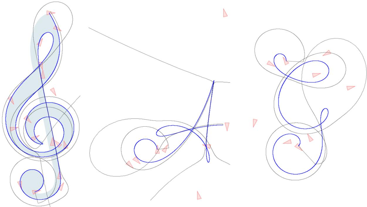
**Figure:** Cubic B-spline refinement applied to 17 control points to partially contour a treble clef. Quartic B-spline refinement applied to 8 control points to form the letter 'A', and 9 control points to form the letter 'G'. ■
