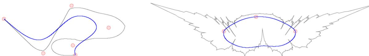
**Figure:** Left, limit curve with curvature comb generated by traditional cubic B-spline subdivision with control points in  $\mathbb{R}^2$ . Right, the non-linear interpolatory scheme by [2005 Malcolm A. Sabin, Neil A. Dodgson] inserts a point by fitting circles through adjacent control points and averaging their radii. The image shows the limit curve generated from three initial control points. The curvature is not smooth. ■
