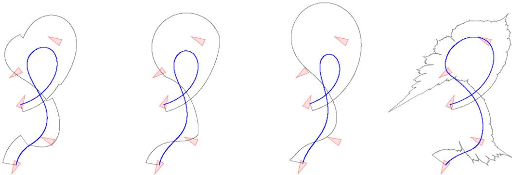
**Figure:** Limit curves and curvature generated by refinement of a sequence of five control points in SE(2) with B-spline rules of order 2–4 as well as the interpolatory 4-point scheme with tensor parameter  $\omega=1/16$ . ■
