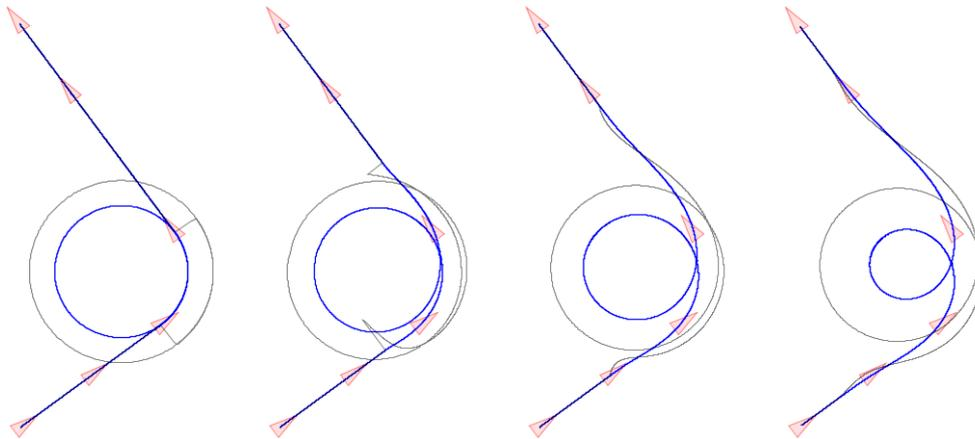
**Figure:** B-spline refinement of order 1–4 applied to a Dubins path that is almost, but not quite, entirely unlike a  $90^\circ$  turn. The angular difference between the 3rd and 4th control point is  $2\pi + \pi/2$ . ■
