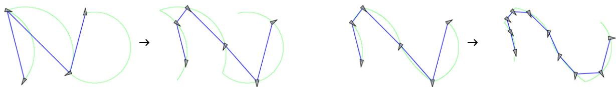
**Figure:** Two rounds of subdivision starting with a sequence of four control points in SE(2). The quadratic B-spline rule inserts two control points at ratios 1/4 and 3/4 along each geodesic segment in green. ■
