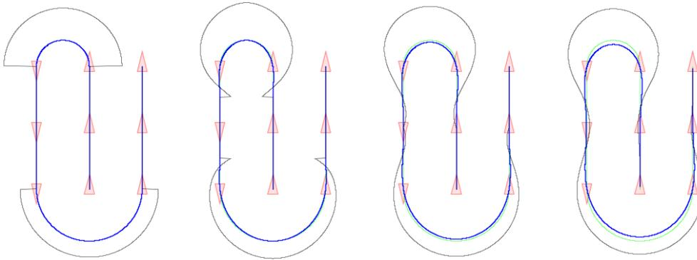
**Figure:** B-spline refinement of order 1–4 of a Dubins path consisting of two U-turns with different radii. The curvature comb of the limit curve projected to  $\mathbb{R}^2$  does not indicate many inflection points when transitioning between a circle and a straight line. ■
