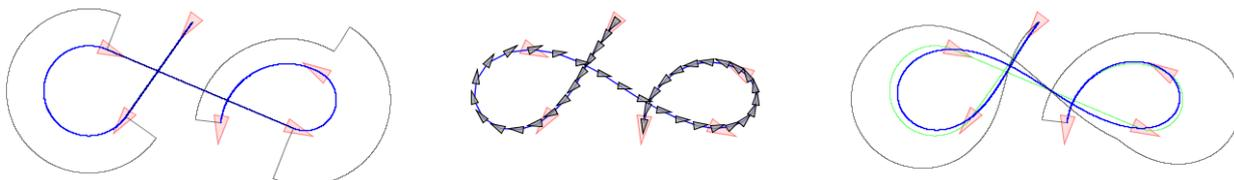
**Figure:** In a Dubins path the heading of a control point in SE(2) matches the tangent of the curve. The curvature of the Dubins path is generally discontinuous as indicated by the curvature comb. The center image shows the refined sequence after 3 rounds of cubic B-spline subdivision in SE(2). To the right is the limit curve with continuous curvature. ■
